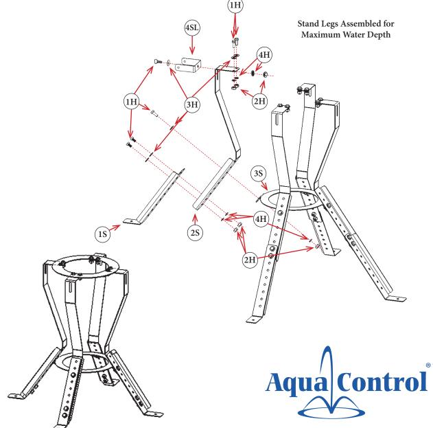
Stand Legs Assembled for Minimum Water Depth
