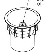
Secure the Nozzle Base to theunit using the bolt that goes through the center hole Finally secure the Center (.6) Nozzle Tip with the plug inserted to the Nozzle base
