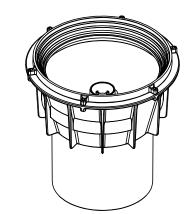
Place the Labyrinth Seal and secure using 6 screws
