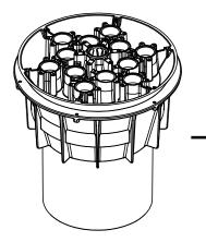
Remove the Nozzle Base by unscrewing the center bolt
