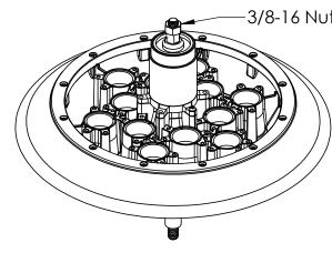
3/8-16 Nut Spin the Module and Base down the Threaded Rod unitl it just begins to make contact with the Labyrinth Seal
